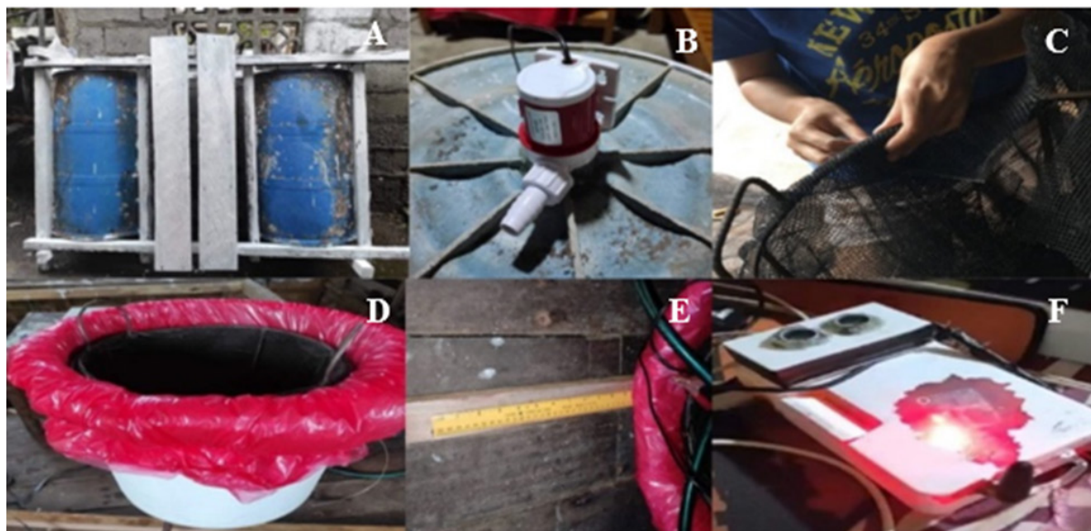
Figure 3. The development phase of SEAGOP: (A) Structuring and painting the floater; (B) mounting the water pump into the catch bin; (C) making of the catch bag; (D) installing the parts of the bin; (E) ensuring the distance from the bin to the sensor; (F) making and calibrating the sensor.
