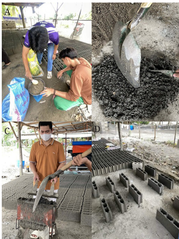
Figure 1. The step-by-step process of producing the Talablocks: (A) Weighing of components; (B) Mixing; (C) Molding; and, (D) Curing.
